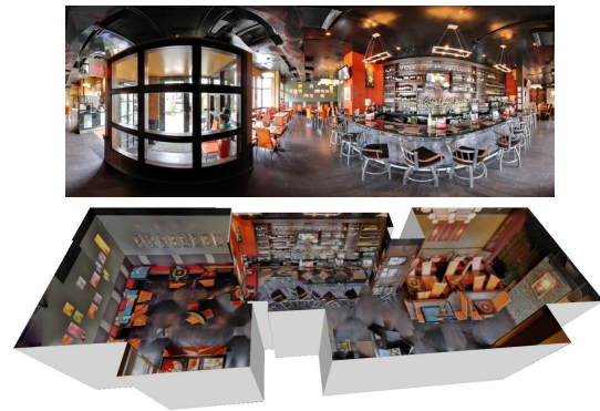
Figure 1. Our system reconstructs high quality texture mapped mesh models of cluttered indoor scenes from panorama images.
