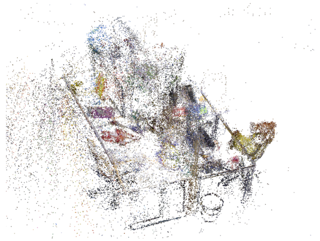
Fig. 9 Ego-motion estimation and mapping results for our proposed algorithm on the fr3/long_office sequence from the TUM RGB-D dataset.
