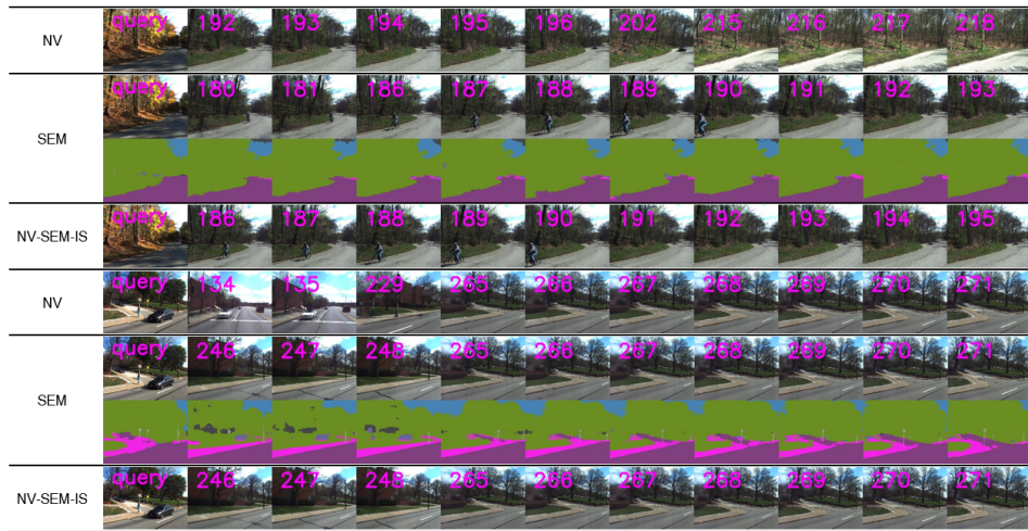
Fig. 8. Candidate images from three localization runs. NV represents localization with NetVLAD retrieval, SEM represents localization with semantic retrieval, and NV-SEM-IS combines the results of NV and SEM by IS. The number in the image is the ID representing its relative position in the database sequence. Improper candidates are filtered out after IS, for example 215, 134.
