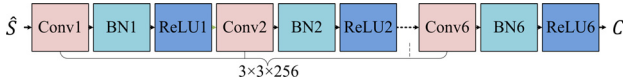
Fig. 4. Architecture of the neural nearest neighbors network. It consists of six convolutional layers with 3 \times 3 kernels, followed by batch normalization and ReLU.
