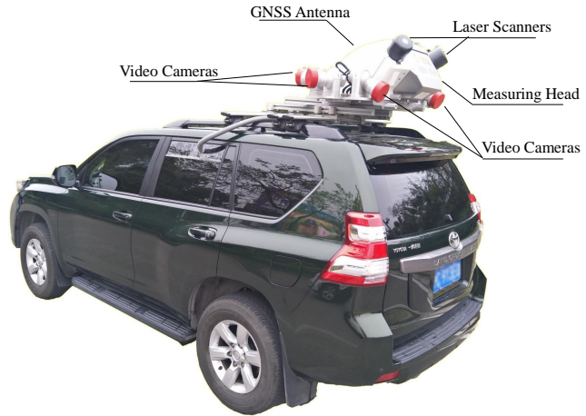
Fig. 2: Acquisition system consists of two laser scanners, up to six video cameras, and a combined IMU/GNSS system.
