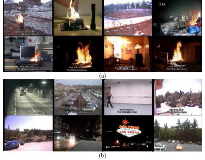
Figure 10. Dataset used in Ko's experiment: Screenshots of video sequences containing (a) actual fires and (b) fire-colored moving objects.
