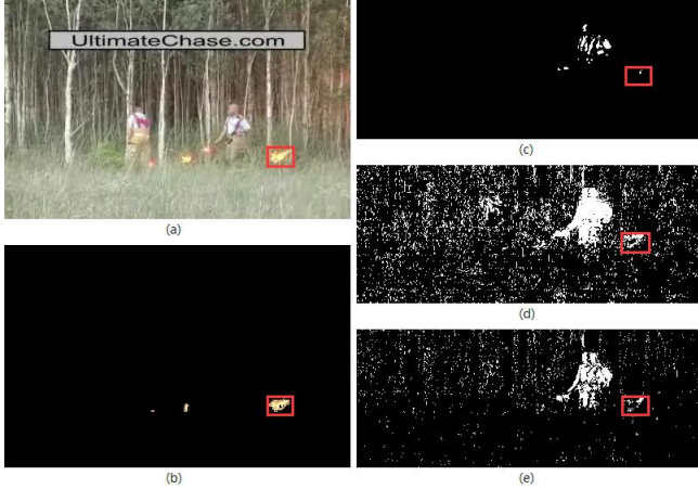
Figure 2. Comparison of three moving detection algorithms. (a) a fire video; (b) our color analysis result; (c-e) the binary images of the detection results of algorithm [14][15][16] respectively.
