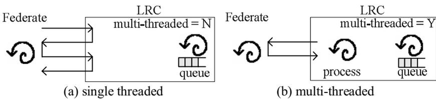
Fig. 6. Implementation of BH RTI Process Model
