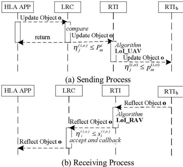
**Fig. 3.** LoI-based Data Delivery Process in BH RTI
