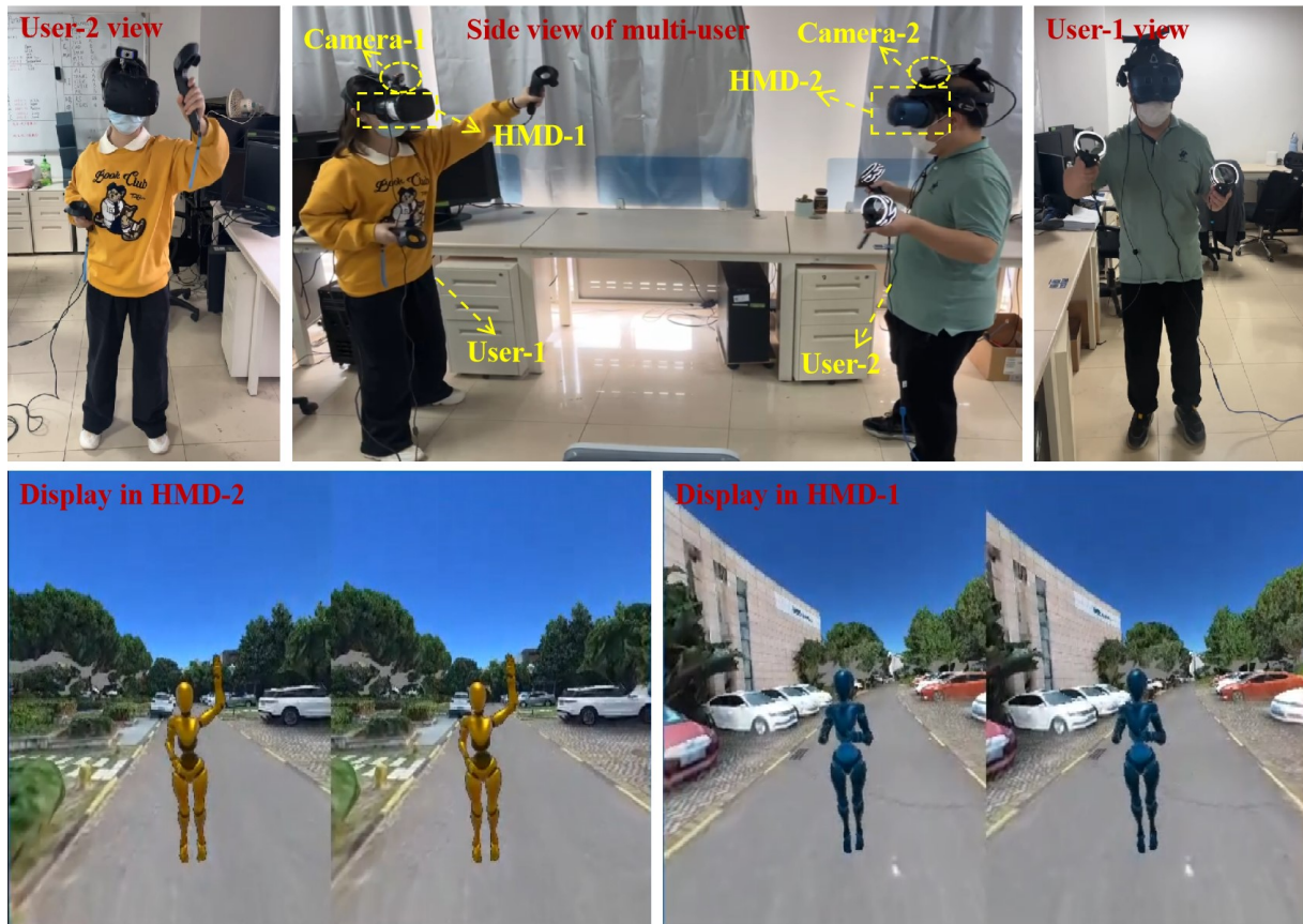
Figure 10 Display in VR devices. In multi-user mode, we use the camera to capture the human body and display the human avatar with pose consistency in the virtual scene.
