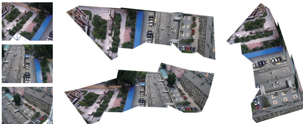
Figure 1 (Color online) Left: simultaneous frames from 3 input videos. Center, right: stitched results rendered from 3 different viewpoints.
