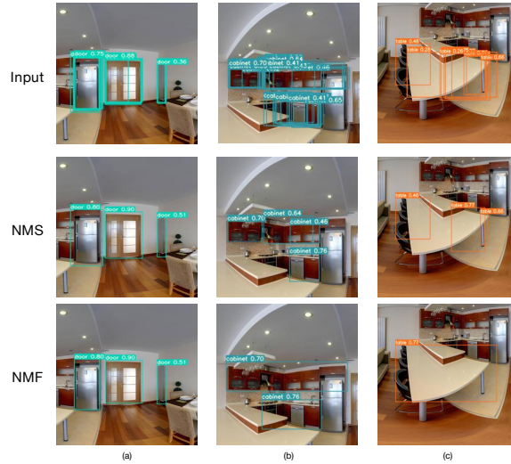
Fig. 5. Qualitative results of the comparison between the non-maximum suppression algorithm and the non-maximum fusion algorithm.
