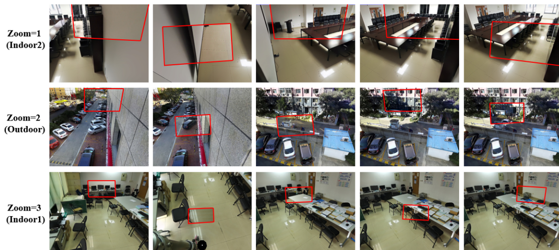
Fig. 7. The result of the proposed PTZ calibration method in real scenes. Red box indicates the real-time video stream from the PTZ camera in real scene. The part outside the red box is from the part view of the half-sphere model.
