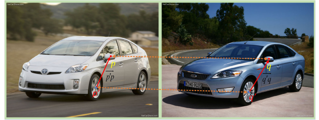
FIGURE 2. The geometric correlations between the positions of salient features. (p, q), (p', q') are two keypoint pairs and the relative distance and orientation between directed line vector pp' and qq' are all intended to be consistency.
