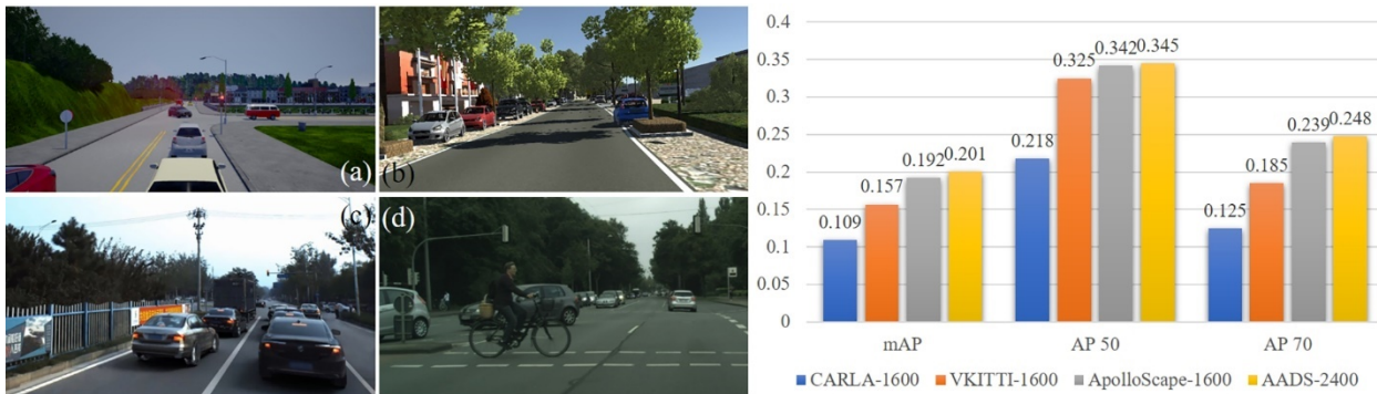
Fig. 5. RGB Image Augmentation Evaluations. The left four images are selected from CARLA (a), VKITTI dataset (b), our AADS-RGB dataset (c), and the testing dataset CityScapes (d), respectively. The right diagram is the evaluation results.
