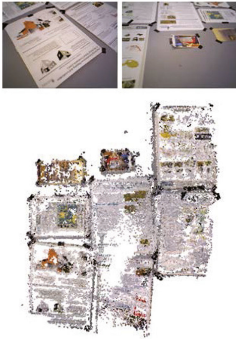
Fig. 11 Reconstruction result of sequence fr3/near [23]. The top shows two frames in the dataset ( left to right frame 235 and frame 830). The bottom shows the semi-dense point cloud reconstruction
