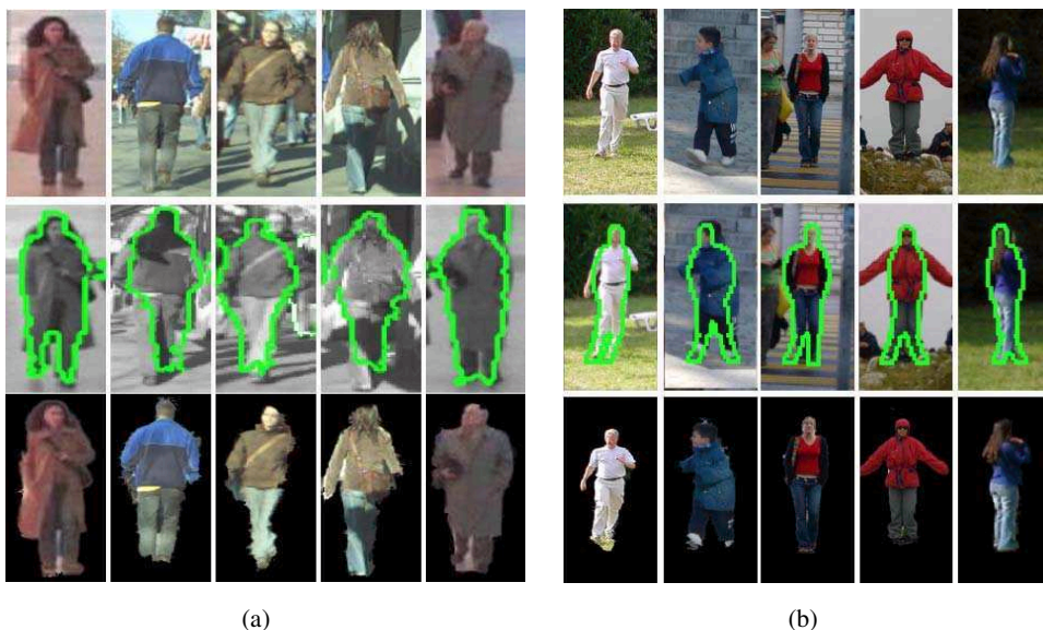
Fig. 7. (Color online) Comparison of segmentation results with Wu et al. and Lin et al. (a) The segmentation results of our method and Wu et al. over the CAVIAR dataset; (b) The segmentation results of our method and Lin et al. over the INRIA dataset. The first row shows the input images from the CAVIAR and INRIA datasets. The second row displays the segmentation results of Wu et al. and Lin et al. , in which the extract silhouettes are displayed in green. The third row shows our results.
